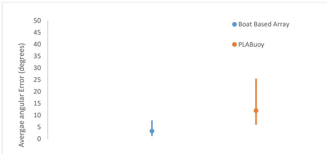
Figure 17. Comparison of error in angle to the pinger for the boat based system and the PLABuoy. In order to minimise errors from GPS systems only ranges >40m were used in angle calculations.
