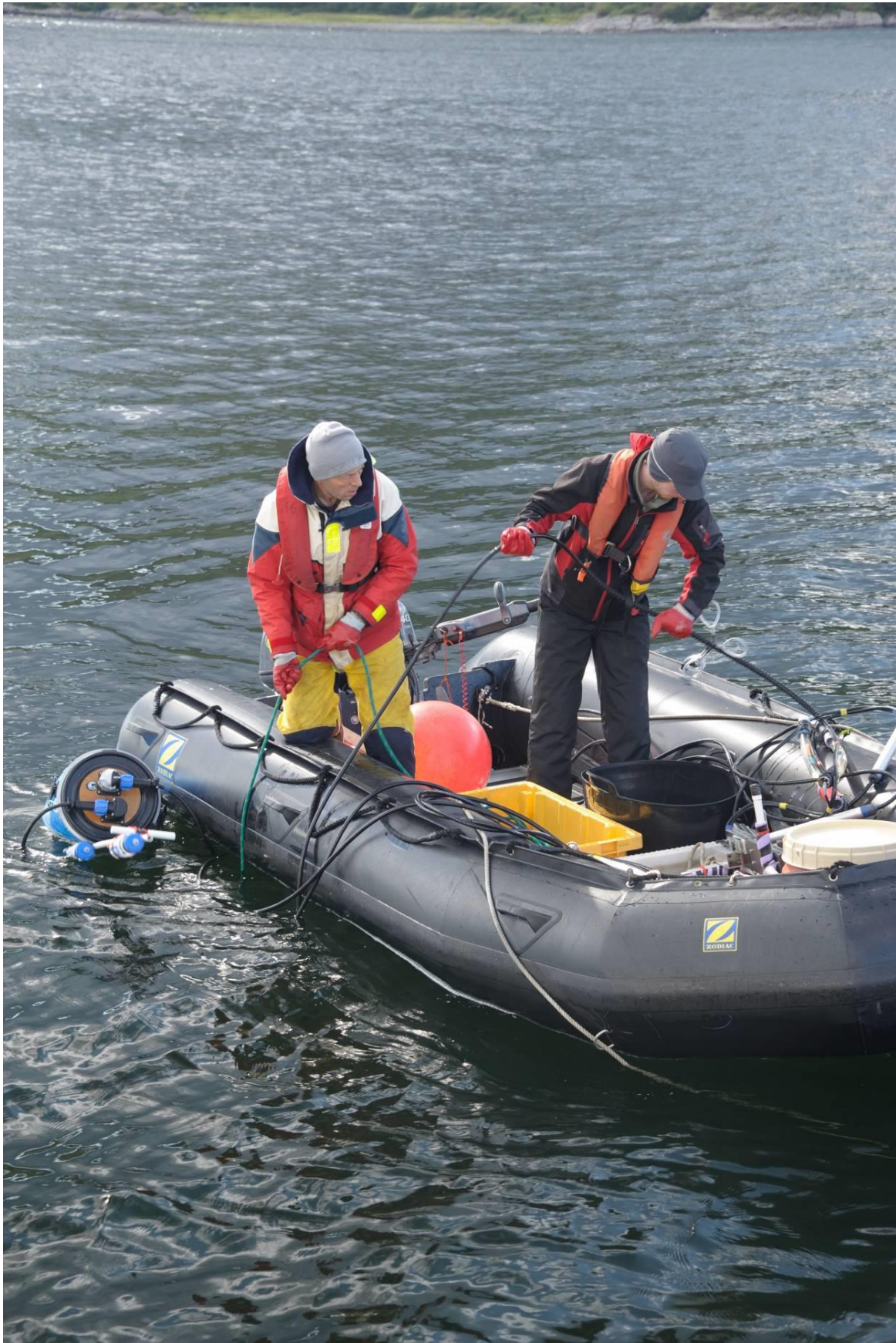
Figure 7. Deploying the PLABuoy. One person (red coat) lowers the weight on a rope. The other flakes out the cable and hydrophones. Once everything is in the water the weight transfers to the hydrophone array allowing it to remain vertical in the water.
