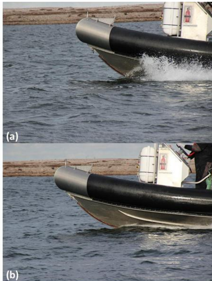
Figure 7. A perpendicular perspective of the blade profile at (a) 6 knots, and (b) 24 knots. Note the elevation of the boat hull with relation to the water surface and the resulting angle of attack of the blade.
