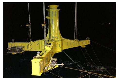
Figure 6. Atlantis TSS being deployed in the Inner Sound (image courtesy of Atlantis Resources Ltd). The HiCUP platform can be seen on the near leg of the TSS, and the PAM and video cameras can be seen towards the centre of each of the TSS legs.
