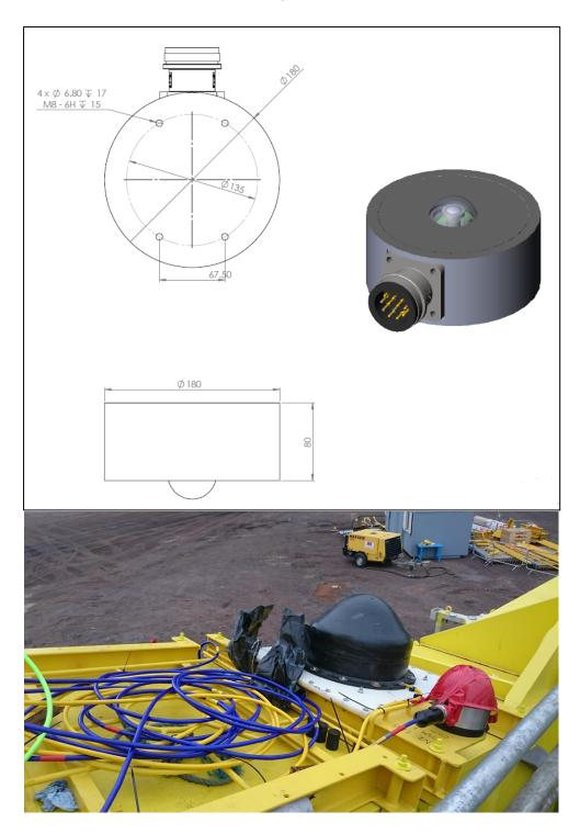
Figure 3. Schematic of the video camera (upper) and a photograph of the PAM module and video camera (lower) mounted on Atlantis AR1500 TSS (under a hard hat to protect the lens during construction).
