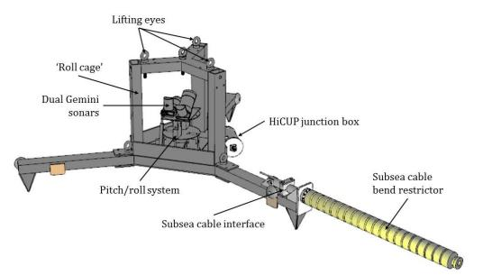
Figure 4. Schematic of the modified HiCUP for the Inner Sound deployment showing the lifting eyes, 'roll cage', dual Gemini sonars mounted on the custom built pitch/roll system, the HiCUP junction box containing the pitch/roll and Gemini control electronics, and the subsea cable interface and bend restrictor.
