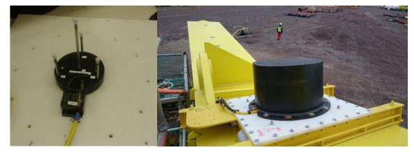
Figure 1. PAM four channel tetrahedral cluster during assembly (left) and mounted within its housing on the Atlantis TSS leg (right).
