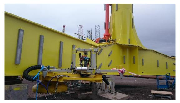
Figure 5. HiCUP mounted on the Atlantis TSS assembly prior to load out and deployment in the Inner Sound.
