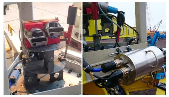
Figure 2. Dual stacked Gemini sonars mounted on the custom built pitch and roll system (left), and the waterproof junction box containing control electronics and power distribution for the pitch and roll system and the Gemini sonars.
