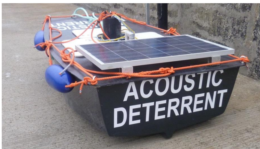
Figure 6. Purpose build fibreglass boat used to deploy an ADD at a salmon bag-net.
