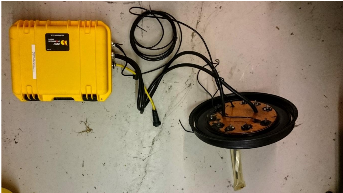
Figure 11. The Peli case was permanently connected to the lid. Future iterations of the PLABuoy would be more practical if plugs were used to connect the Peli case to the lid.
