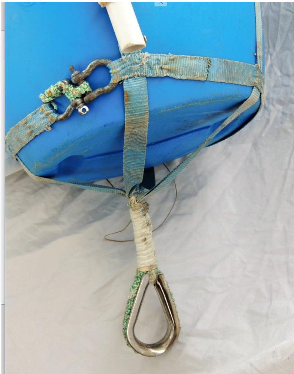
Figure 5 Vertical straps in the “girdle” are brought together and pass around a stainless thimble below the tub to provide the main attachment point for the vertical array
