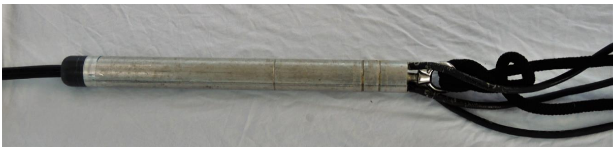
Figure 14 The lower termination of the vertical array cable.
