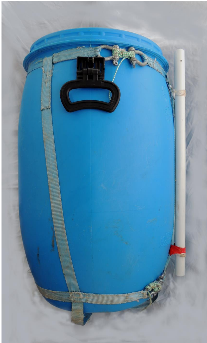
Figure 3 Drum with webbing “girdle”. The white plastic tube to the right serves as a holder for a short “mast” that supported a flag and a GPS logger.
