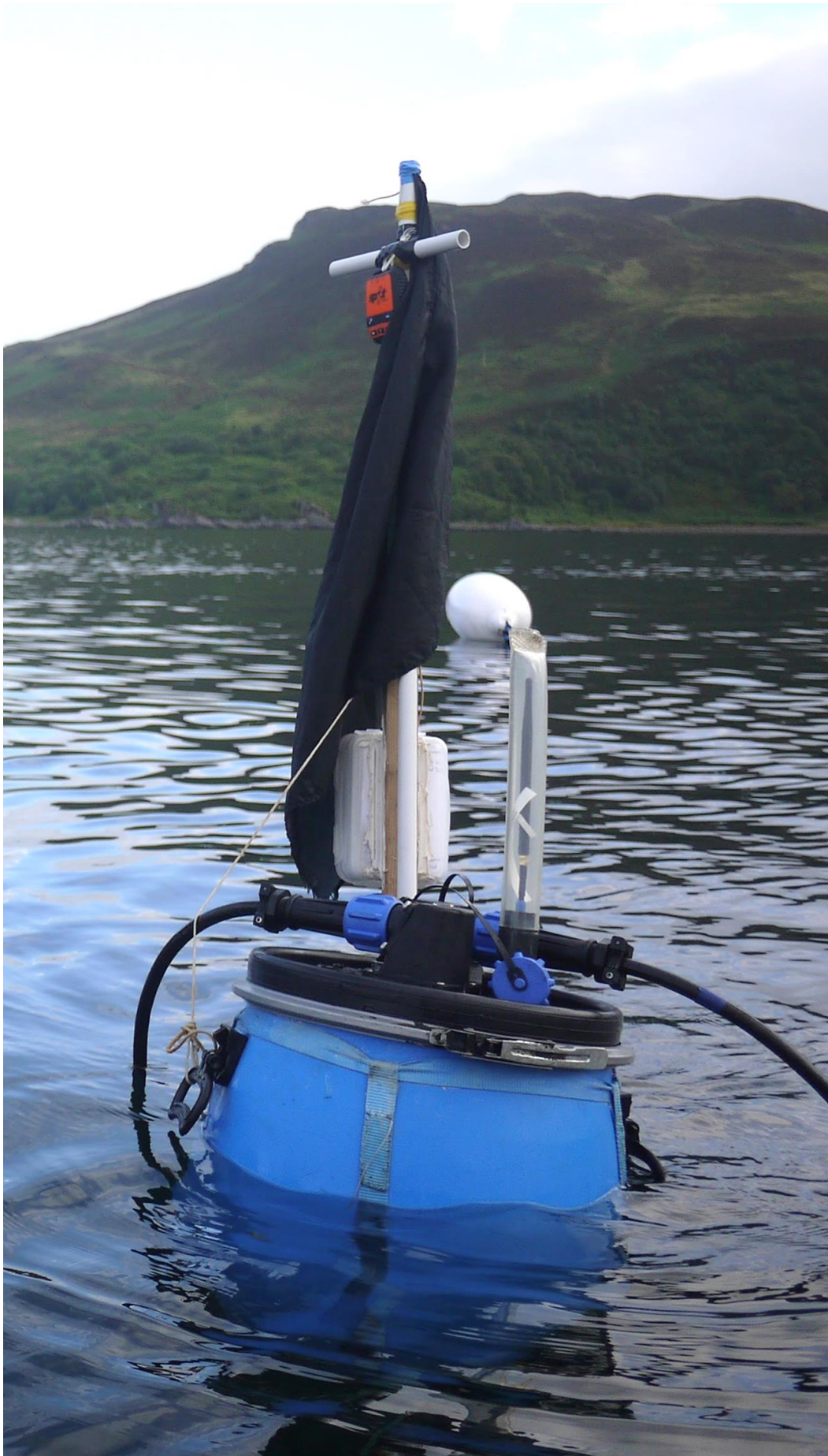
Figure 10. The lid of the PLABuoy. This contained connections for the electronics and hydrophones array and a GPS and Wi-Fi aerial.
