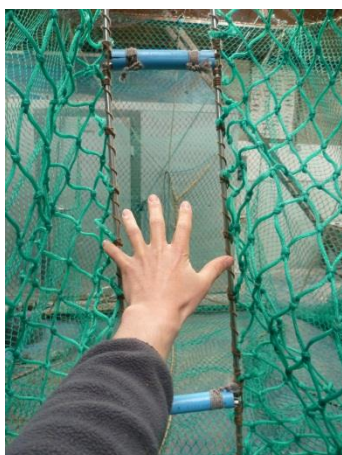
Figure 7. A close-up view of the entrance to the inner chamber of a modified salmon bag-net illustrating the size and ridged steel framed entrance
