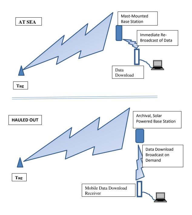
Figure 1. Schematic of telemetry system showing at sea and shore based data download options
