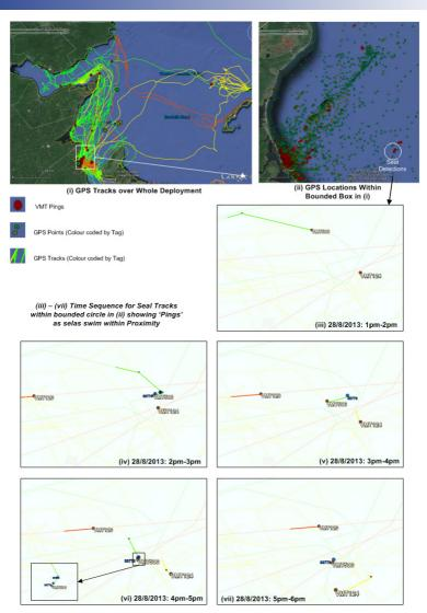
Figure 4: (i) GPS tracks from the whole deployment; (ii) GPS locations within rectangular box, showing individual GPS locations; (iii - vii) Hourly time sequence focussing on a small area where three seals, numbered 124, 126 & 506 swim within close proximity. The navy blue 'target' symbols indicate the locations where the VMT-tagged seal has detected the presence of another.
