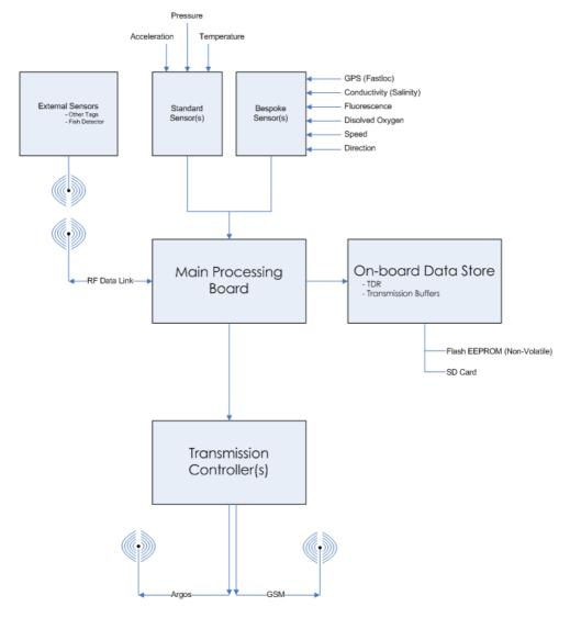
Figure 1. Schematic diagram of tag architecture and optional sensors and data channels
