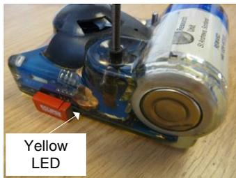
A rather faint **yellow** LED mounted along the edge of the PCB will flash approximately once every 4 seconds. If it doesn't flash, remove magnet and try again.
